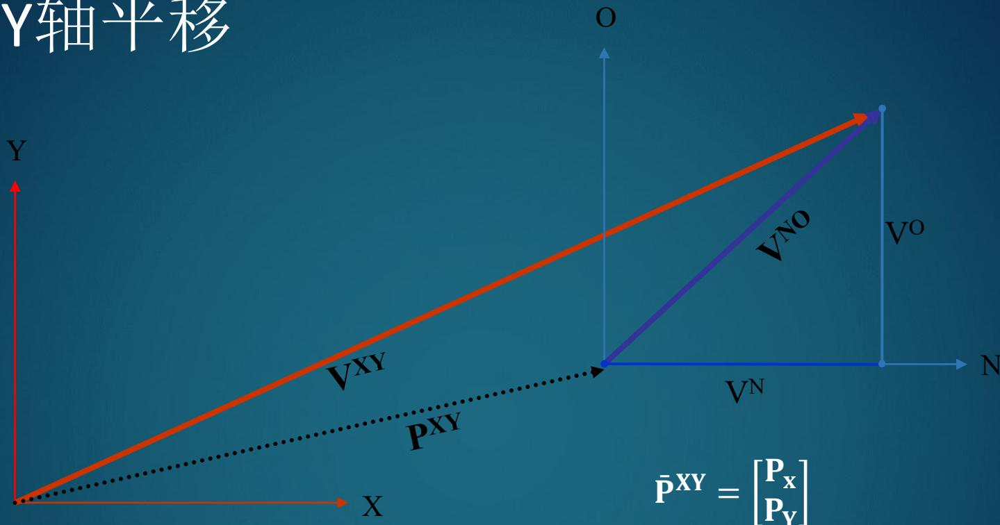
$$\bar{V}^{XY} = \bar{P} + \bar{V}^{NO} = \begin{bmatrix} P_x + V^N \\ P_y + V^O \end{bmatrix}$$
