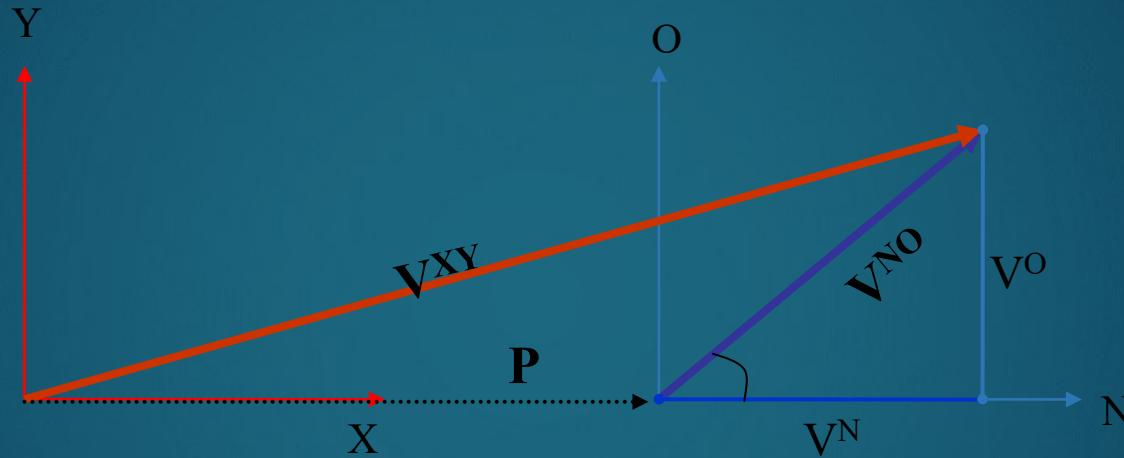
$$\bar{v}^{XY} = \begin{bmatrix} P_X + V^N \\ V^O \end{bmatrix} = \bar{P} + \bar{v}^{NO}$$
