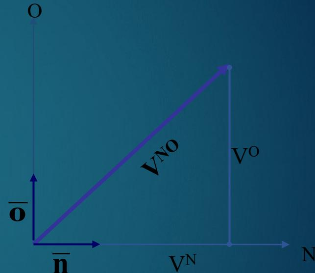
$$\bar{V}^{NO} = \begin{bmatrix} V^N \\ V^O \end{bmatrix} = \begin{bmatrix} \|V^{NO}\| \cos\theta \\ \|V^{NO}\| \sin\theta \end{bmatrix} = \begin{bmatrix} \|V^{NO}\| \cos\theta \\ \|V^{NO}\| \cos(90 - \theta) \end{bmatrix} = \begin{bmatrix} \bar{V}^{NO} \cdot \bar{n} \\ \bar{V}^{NO} \cdot \bar{o} \end{bmatrix}$$
